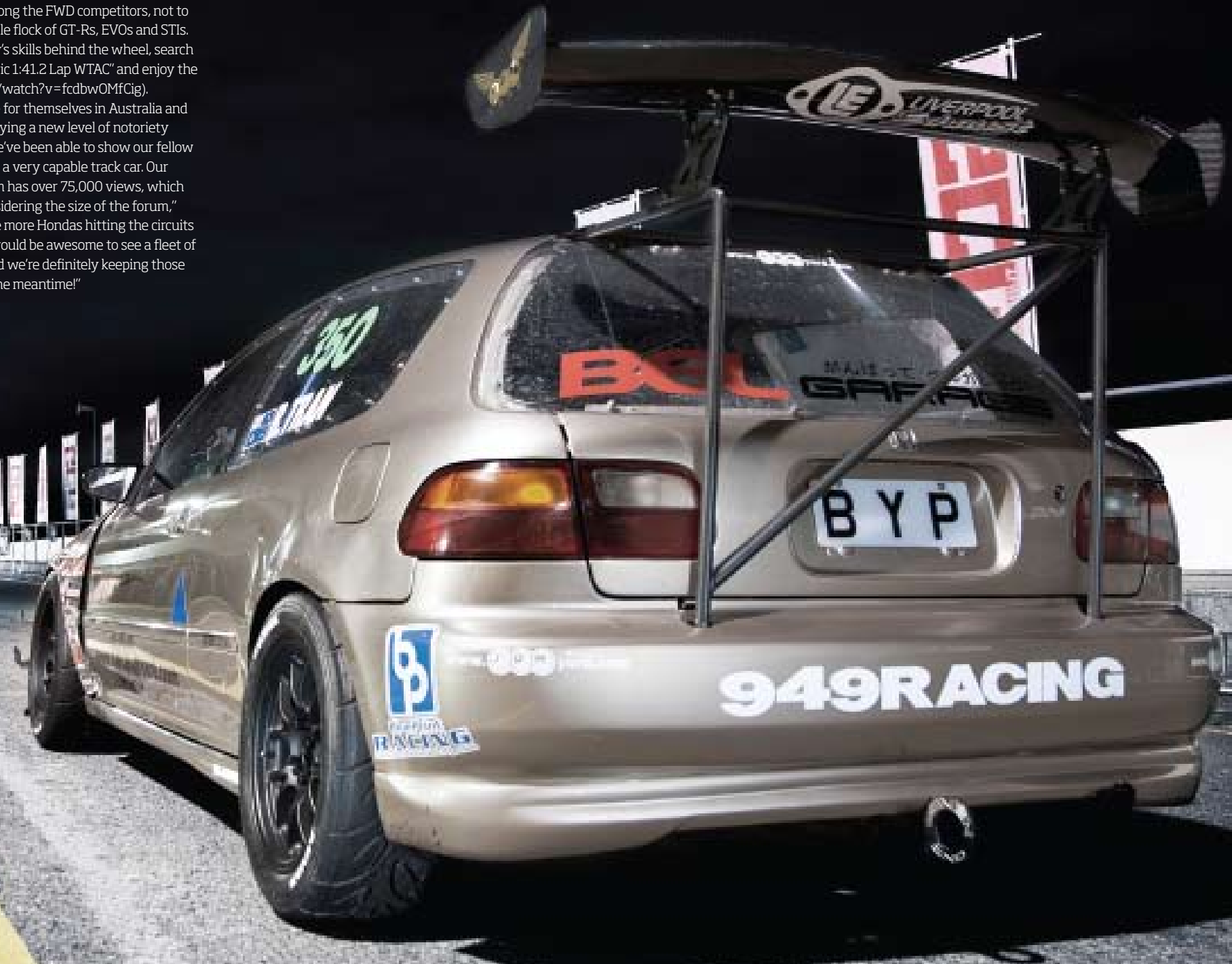
Exterior BYP custom front splitter, canards, rear spoiler brackets & generic wing; Spoon style mirrors, flared, rolled & spaced front fenders; Lexan windows
