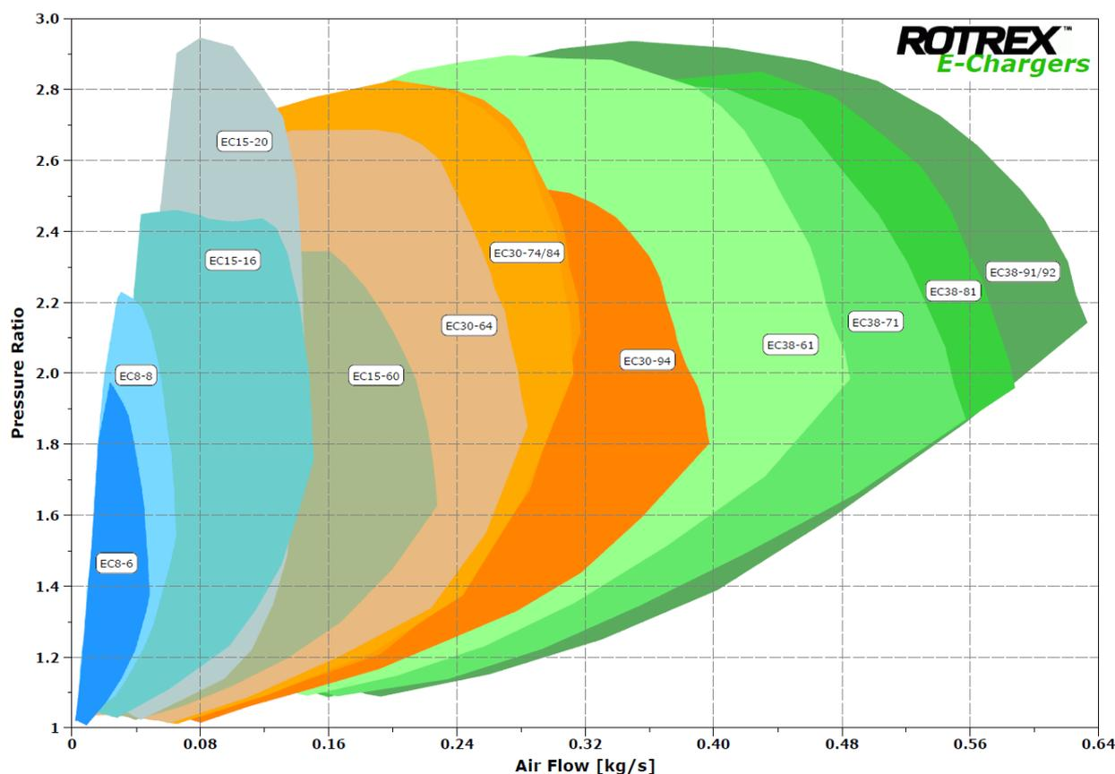
(The Rotrex E-charger range now covers an immense span of air flows with the introduction of the EC30 and EC38)
